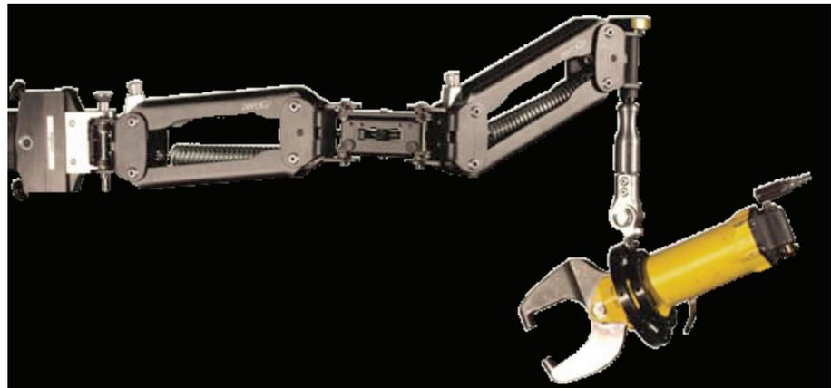
position and angle that workers need. Providing up to four axes of motion, the gimbals can be attached and removed quickly.
